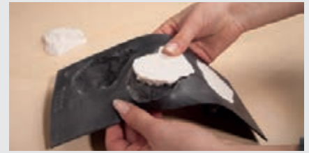
After hardening, the individual rocks are carefully pushed out of the mould.
