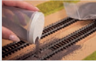
The ballast is now loosely scattered. The NOCH Shaker (ref. 08099) is very useful for this.
