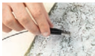
The crocodile clip (counter-pole) is fastened near the surface where the grass is to be applied.
