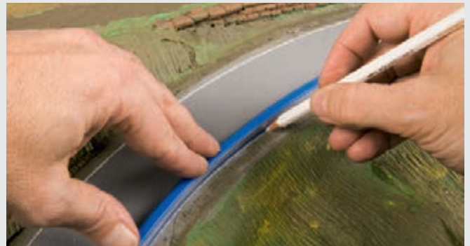
Customised edge lines can be drawn with the Curved Ruler and the Street Marking Pencil.
