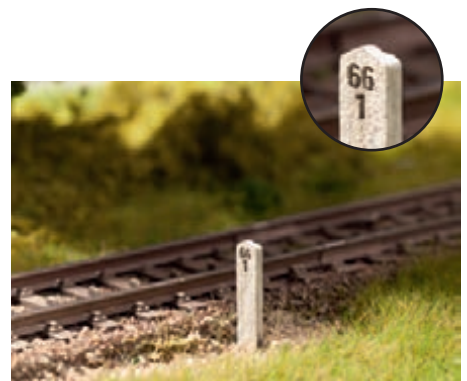
H0 14300 Milestones 20 milestones in 100 metre steps. Milestones can be mainly found along non-electrified branch lines. The upper number informs the engine driver about the track section and the lower one about the 100 metre mark. Mileage allocation randomly selected in the package.
