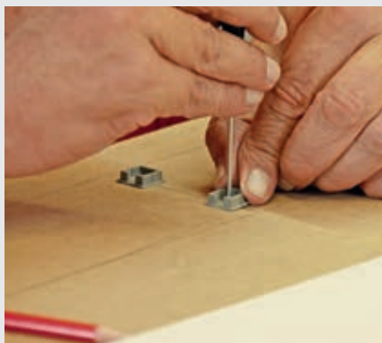
2. At the joins of the rail routes, floor slabs for the pillars are screwed on.
