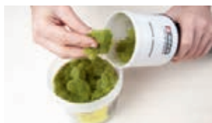
The grass fibres are loaded into the grass container. Different lengths and colours can thus be mixed together.
